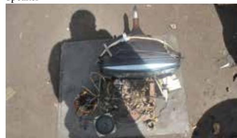
The CRT and Disassembled Parts
