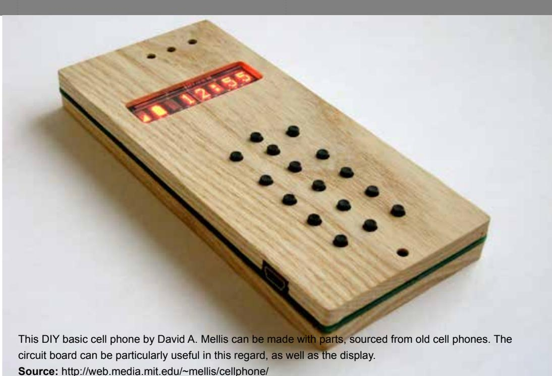
This DIY basic cell phone by David A. Mellis can be made with parts, sourced from old cell phones. The circuit board can be particularly useful in this regard, as well as the display.
