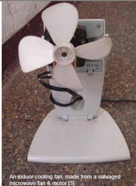
An indoor cooling fan, made from a salvaged microwave fan & motor [3]
