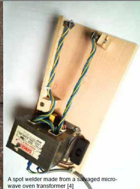
A spot welder made from a salvaged microwave oven transformer [4]
